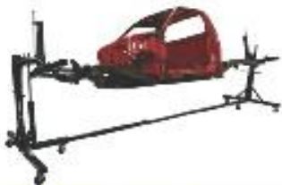
CAR ROTISSERIE TL1.3ROT 1.3 TON/1300 KG CAPACITY
