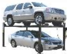
4 POST PARKING HOIST TL3.6PH-S 3.6 TON/3600 KG CAPACITY
