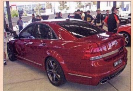
One of the last, a 2016 HSV Statesman Grange SV, powered by a 462hp 6.2 litre V8.
